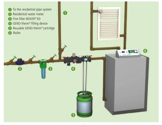
Installation example of a heating system
